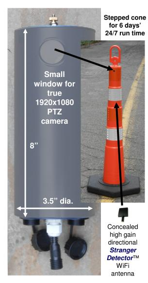
The *Cylindrical Cellular Covert Smart uPTZ Camera* is far more than a camera. It is a versatile and powerful <u>labor-saving system</u> that is mounted inside the top of the *Private Investigator's Apprentice*. It is 3.5"D x 8"L, 3# and mimics 3" PVC conduit. It can be used in the cone, exposed or in an outer rectangular or cylindrical, horizontal or vertical housing, with orientation chosen in software. Cell antenna not shown. Appearance varies.
